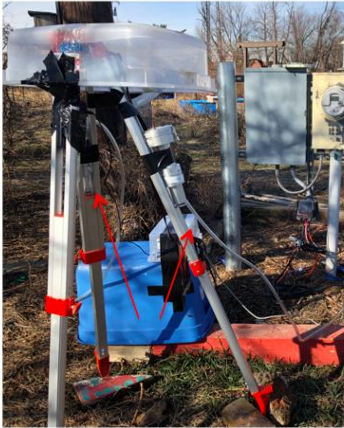
Impactors on Tripod in the middle of Filbert Garden, next to power source
