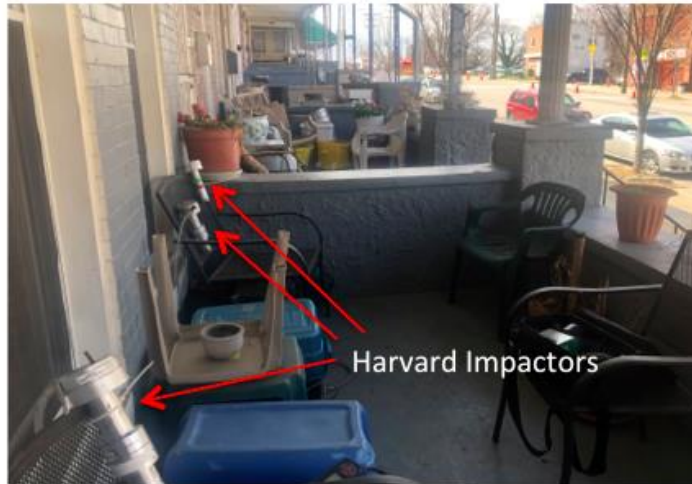
Harvard Impactors zip-tied to chairs on Annapolis Road, 0.7 miles from the trash incinerator
